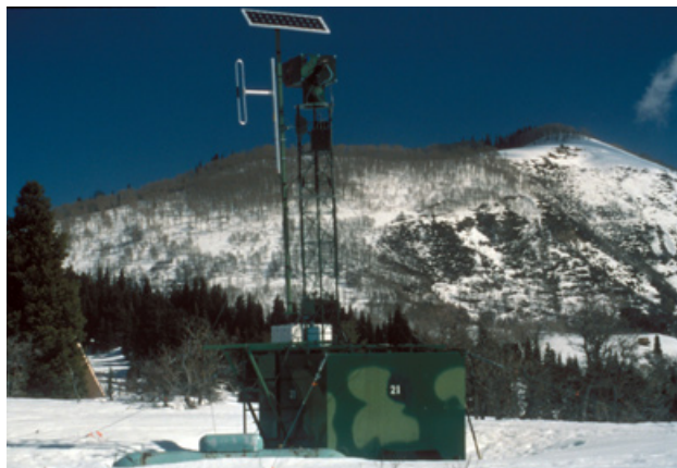
A ground generator used for cloud seeding in the Western U.S.
